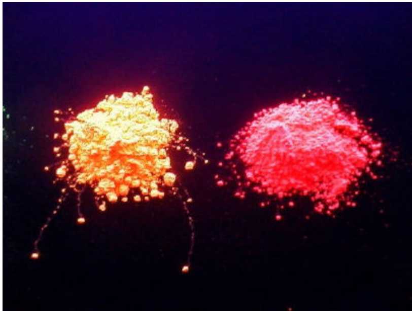
Fluorescent coatings will be applied to the tracer material to allow identification of particles in seabed sediment samples.
