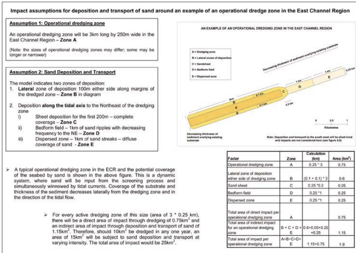
Based on reasoned assumptions presented in section 4 (chapter 5 of the REA), the following model has been developed. The conceptual model has been developed to quantify the potential effects of the impact of dredging due to deposition and mobilisation of screened sediment.
