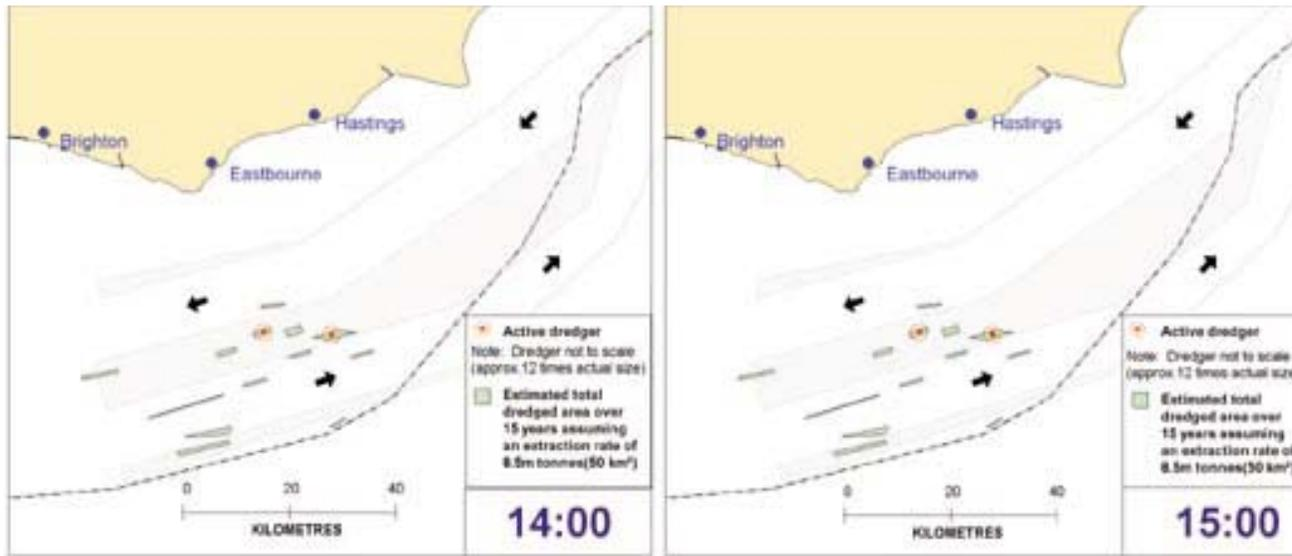
This plans shows dredger occupancy at 2pm and 3pm on a typical day assuming production of 8.5 million tonnes pa. Typically, an average of five dredgers will operate in the ECR each day and it is likely that there will be a six-hour interval without activity. When dredging concurrently, it is likely that dredgers will be separated by 5 to 10 km.
